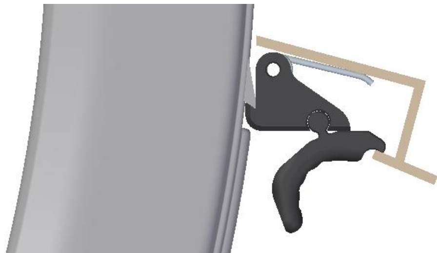
Figure 3: INSTALLATION IN THE STOCK – correct placement
